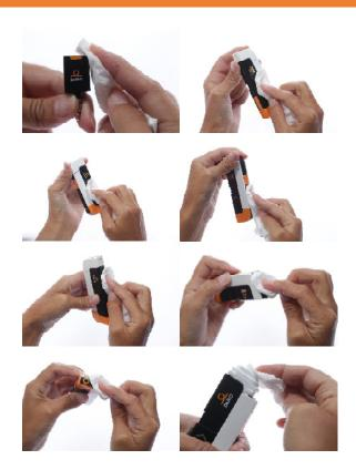
To ensure effective disinfection, let the solution sit on the meter, housing, orange lancet cover, and white cartridge cover for at least two (2) minutes. Allow the meter, housing, orange lancet cover, white cartridge cover and cartridge cap to completely dry before use. Wipe off any remaining residues with a clean, soft, and dry paper cloth.
